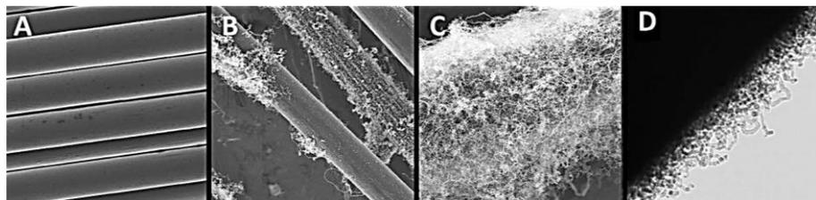
**Figure 1** | (A) CF as received from the manufacturer. (B) No potential difference applied to CF - shows damage through catalyst pitting and poor nanotube coverage. (C) Potential difference applied to CF - shows no CF damage, promoted nanotube synthesis and superior coverage. (D) applied potential difference to the carbon fibre in continuous arrangement, showing nanotube coverage.
