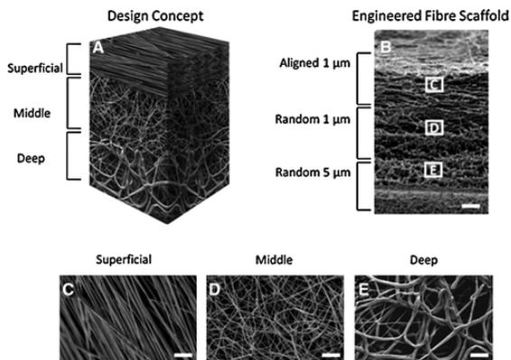
Zonal fiber mechanical properties can be fabricated by the proposed technology in a continuous scaffold. The diagram (A) illustrates the zonal placement of varying fiber zones and the resultant electron microscopy images of the bulk anisotropic scaffold (B) and the varying fibers of aligned (C), randomly oriented (D), or randomly oriented fibers throughout the scaffold (E). Scale bar = 100 μm in (B); 10 μm in (C–E).
